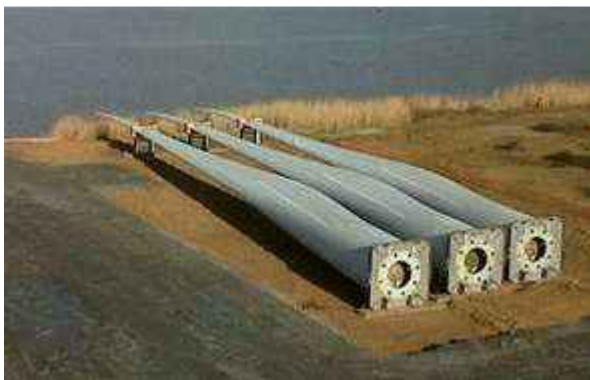
Figure 7 – Pales de l'éolienne Haliade 150 a vant installation (source Alstom)
